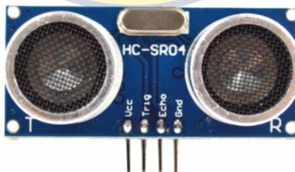
Gambar 2.5 Sensor Ultrasonik (HC-SR04)
