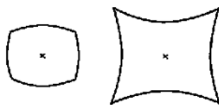
Fig. 3 Effect of radial distortion on image geometry
