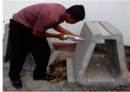
Fig. 14: Pressure Hammer Test Precast Foundation Model
