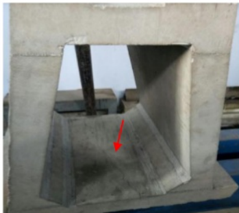
Fig.13: Side wall – bottom crack foundation
