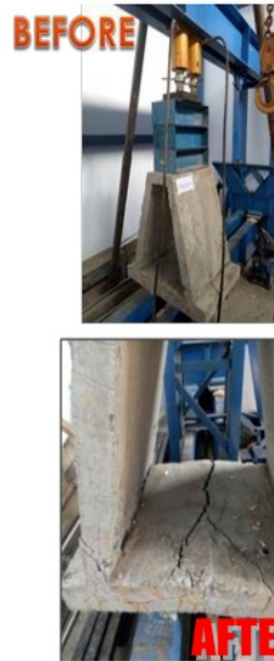
Fig. 4: Precast foundation design and pressure test [1]
