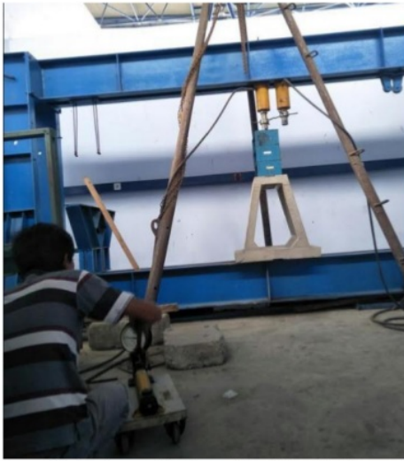
Fig.12: Pressure Test Precast Foundation Models
