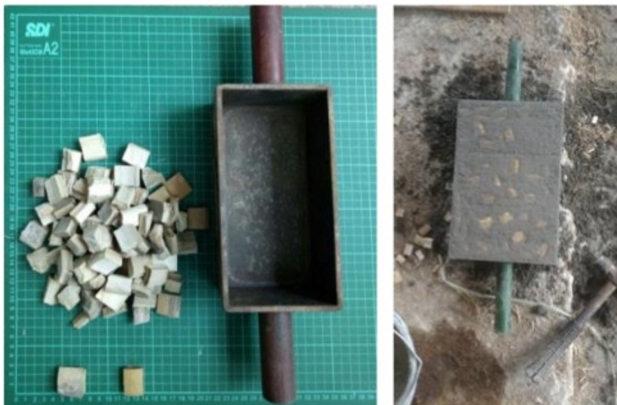
Gambar 6.7. Paving bermaterial Bambu
