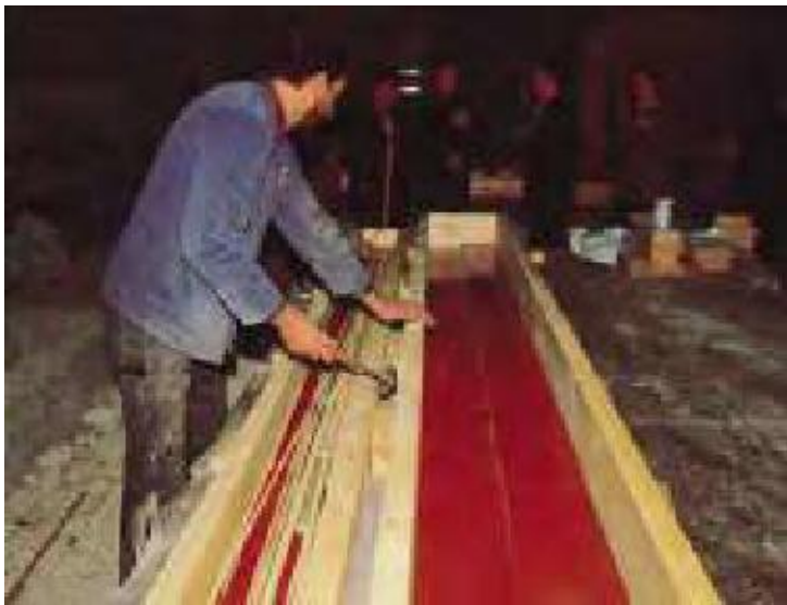
Gambar 1.9 Cetakan Precast dari kayu (Sumber: Architecture In Precast Concrete, Building and Construction Authority, December 1999, ISBN 9971-88-707-X )
