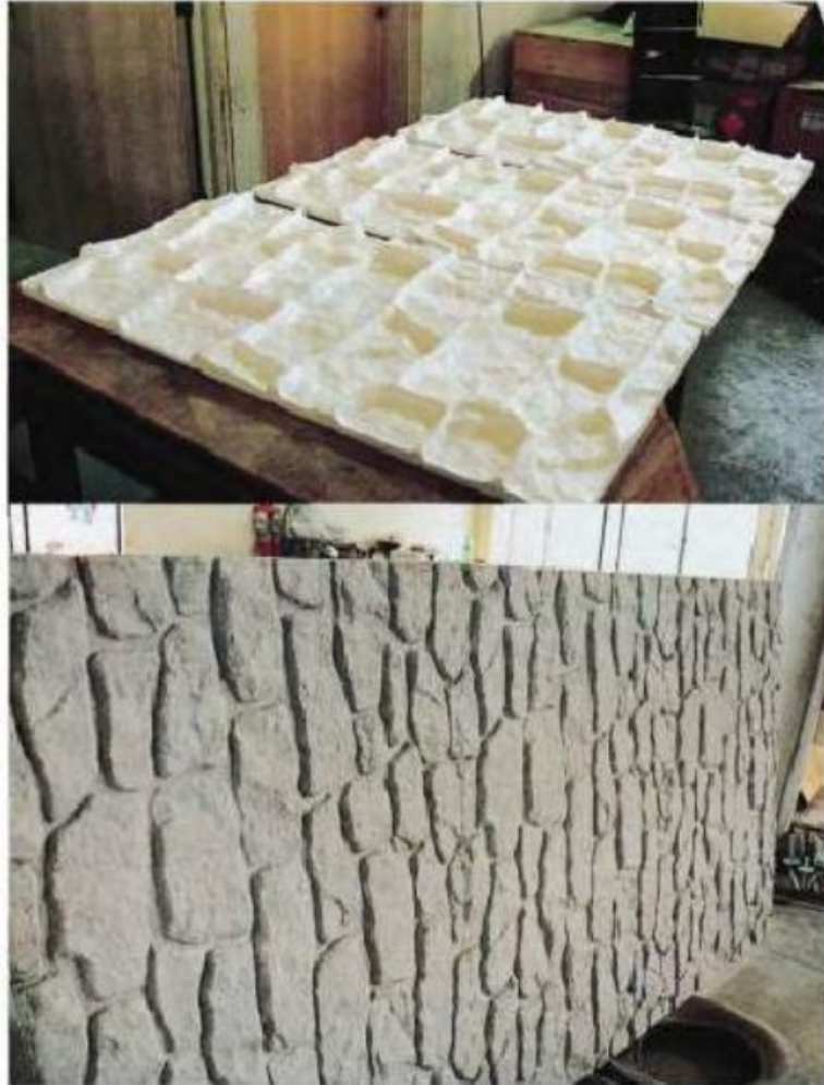
A stone-effect precast wall using polystyrene mould technique which has a range of surfaces to choose from and is available from local precasters
