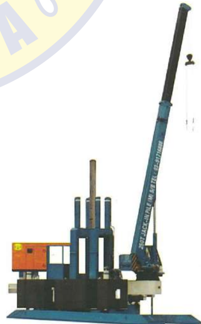
250 Tons Hydraulic Jack-in machines with crane
