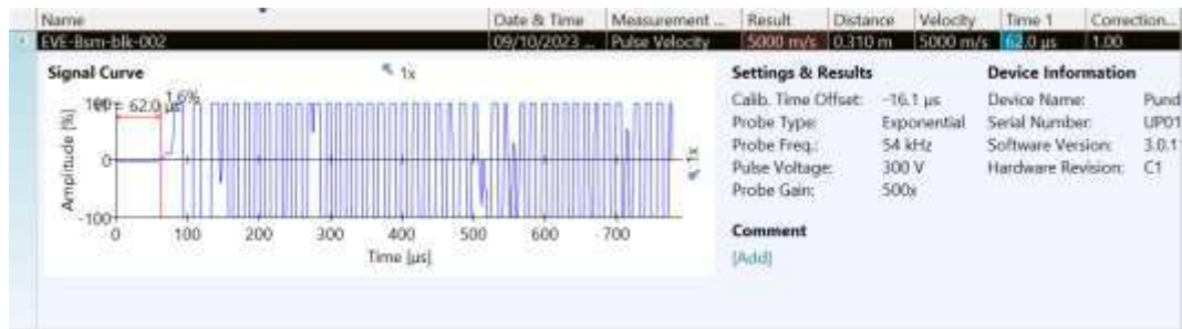
Gambar 4. 26 Hasil Grafik Pengujian UPV Direct Elemen Balok, V=5000 m/s (Excellent)
