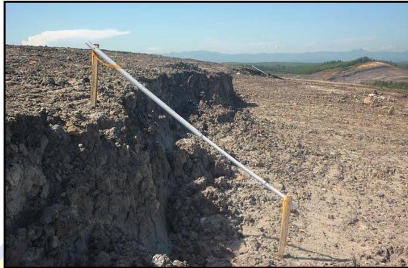
**Gambar 2-21.** Crackmeter (R. Musa, 2012)
