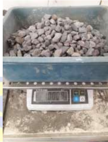
Proses penimbangan agregat kasar
