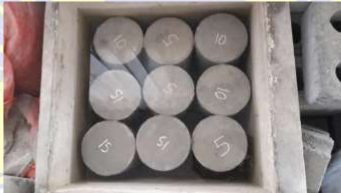
Proses curing beton
