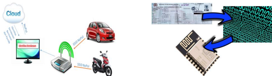
Figure 10.3: System Block Diagram and Vehicle Identity Embedded to ESP8266
