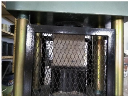
Figure 2. Compressive strength testing process in test objects.
