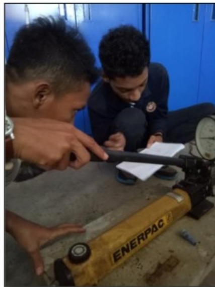
Gambar 7.8 Pencatatan Dial Pressure Pump Uji Tekan
