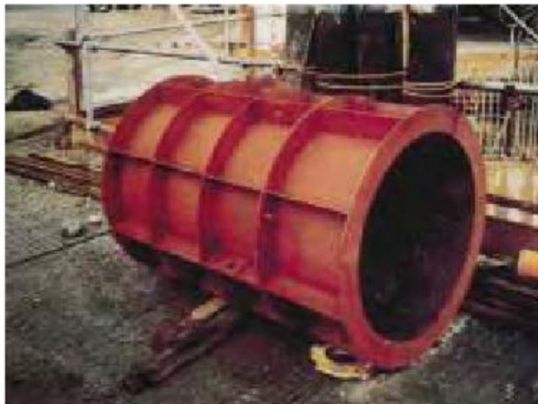
Gambar 1.8 Cetakan Kolom Bulat Precast (Sumber: Architecture In Precast Concrete, Building and Construction Authority, December 1999, ISBN 9971-88-707-X )
