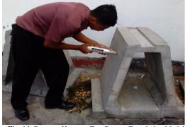
Fig. 14: Pressure Hammer Test Precast Foundation Model
