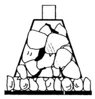
Fig. 2: Typical stone foundation [8]
