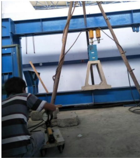
Fig.12: Pressure Test Precast Foundation Models
