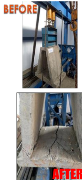
Fig. 4: Precast foundation design and pressure test [1]
