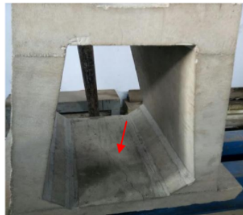
Fig.13: Side wall – bottom crack foundation
