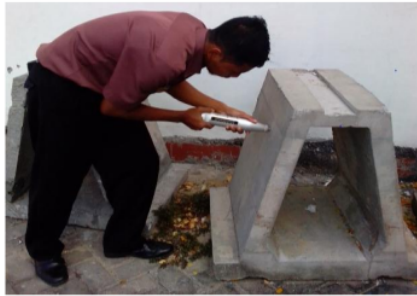
Fig. 14: Pressure Hammer Test Precast Foundation Model
